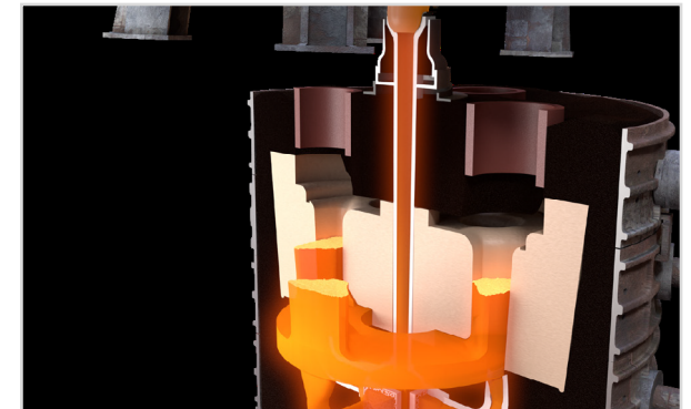
Non-turbulent flow with HOLLOTEX Shroud application
