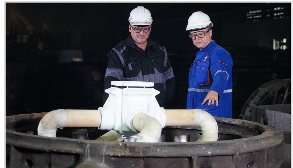
HOLLOTEX Shroud Filter Box during moulding
